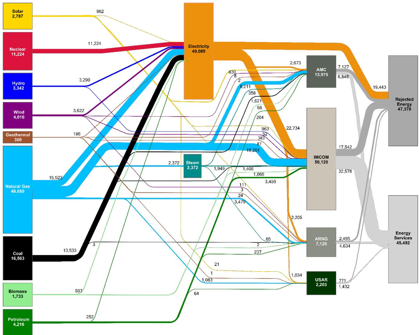
Figure 1: Army Installation Energy Sankey Diagram
