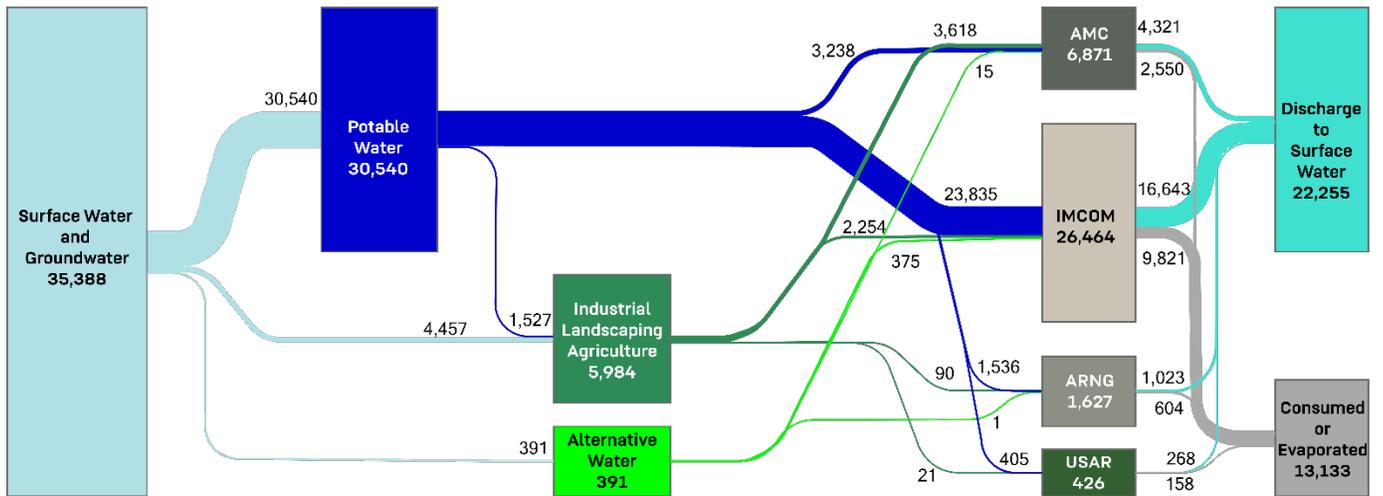
**Figure 2: Army Installation Water Sankey Diagram**
