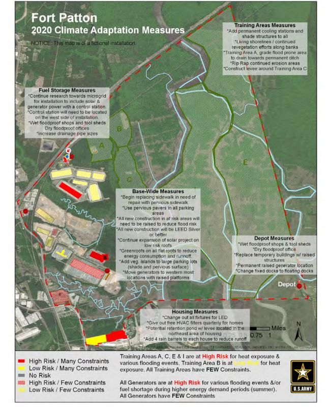
Figure 18: Example Installation Profile Map with the GIS layer produced during Step 4 showing concepts of climate adaptation measures
