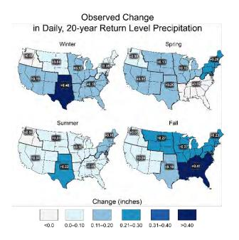
Figure A.8: Observed changes in precipitation for the 1 day, 20-year return interval storm for CONUS between 1948 and 2015. (Easterling et al. 2017: Fig 7.2)
