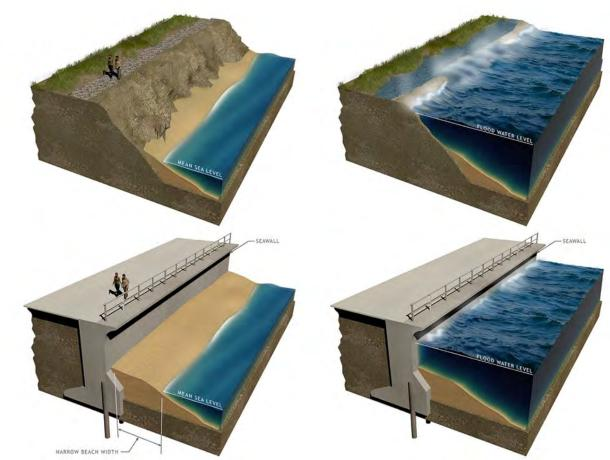
Figure C.7: Example of how a sea wall provides coastal resilience under tide-influenced flooding (left) and hurricane or extratropical storms (right) (after USACE 2015)
