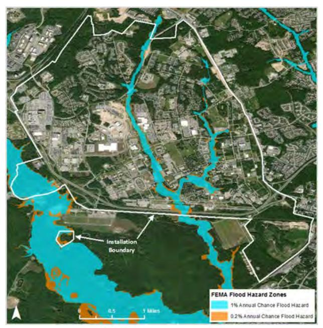
Figure A.11: Example of flood extent mapping, showing the area of an installation impacted by the 1% and 0.2% AEP
