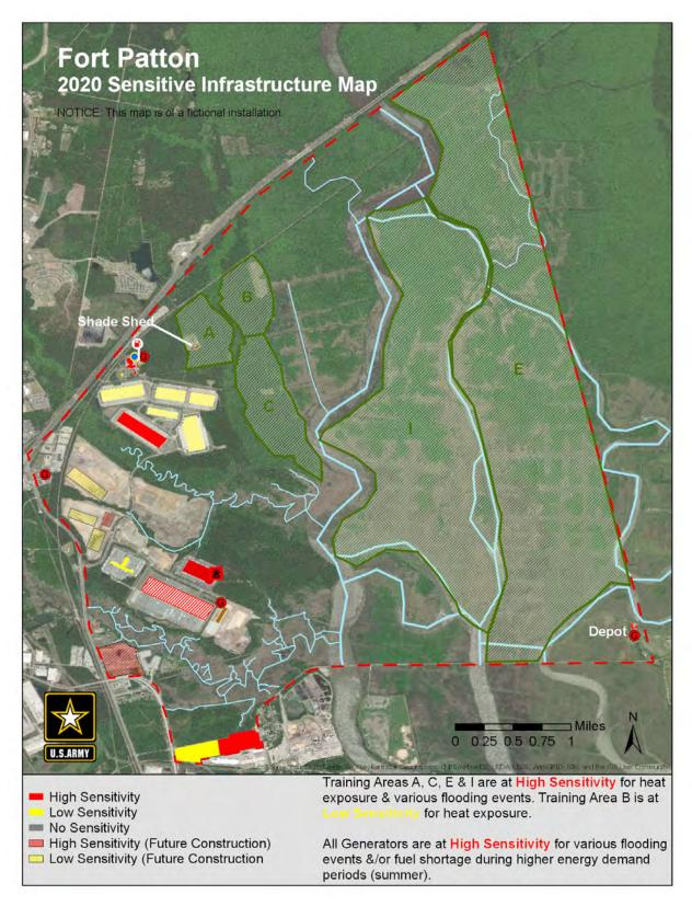
Figure 14: Example Installation Profile Map with the sensitivity color-coding GIS layer produced during Step 3
