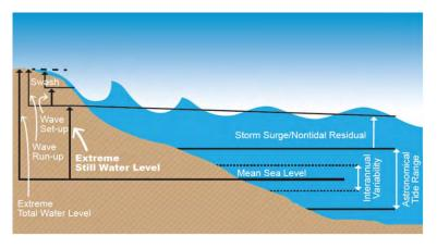
Figure A.5: Schematic of major components of coastal water levels
