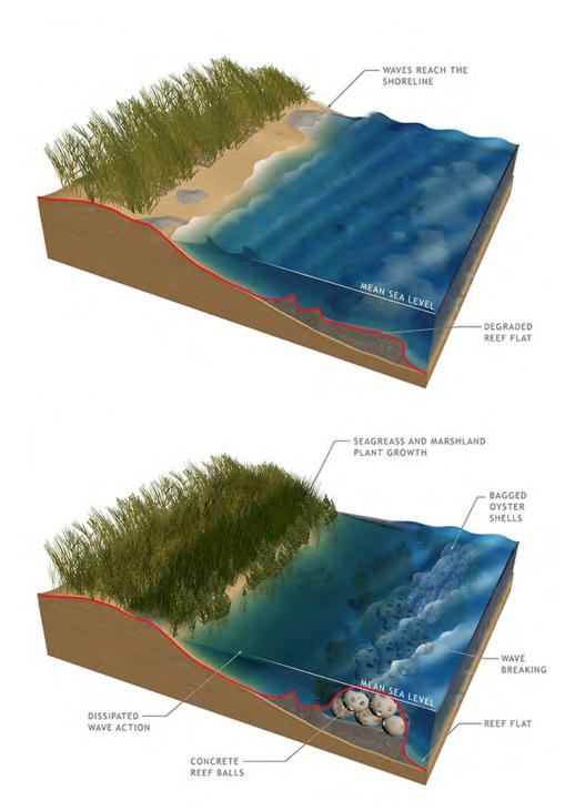
Figure C.8: Establishing artificial reefs (bottom) can reduce wave damage along the coastline, allowing for reestablishment of coastal and submerged aquatic vegetation, and reducing wave erosion (after USACE 2015)
