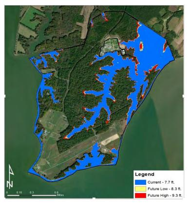
Figure A.6: Coastal inundation extent for a typical coastal installation
