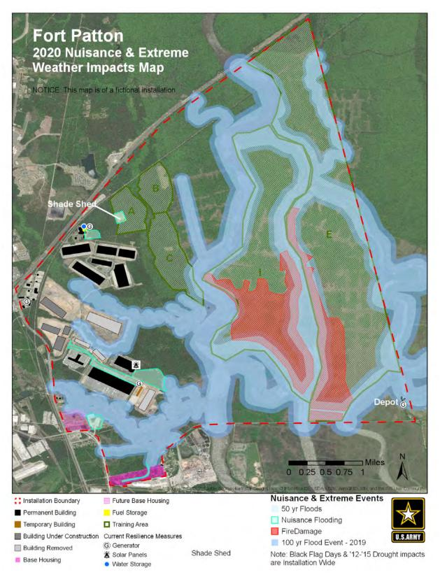
Figure 10: Example Nuisance and Extreme Weather Profile Map. The map includes the extreme weather and the previously mapped nuisance weather impacts GIS layers produced during Step 2a
